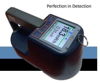
**The IC3** is a battery operated, auto ranging, portable ion chamber survey meter designed for highly stable and accurate measurement of dose rates and integrated dose of gamma, x-ray and beta radiation.
