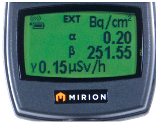
Display with Alpha/Beta Probe
