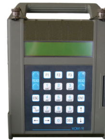
Portable reader/recorder for NBC dosimetry XOM/T
